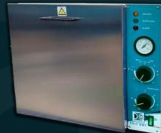
The sterilizers of HOT DRY series use the principle of heat transfer. An armored electrical resistance allows the air, within the sterilization chamber, to reach a uniform temperature (that can range from 160 to 180°C), and comes into contact with tools allows a complete and effective sterilization.
